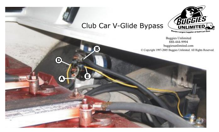
The other end of the cable marked (A) is connected to the post marked (F).
